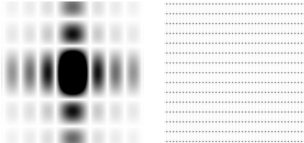
(The Fourier transforms of the motif and the lattice are multiplied to obtain the Fourier transform of the crystal structure)
