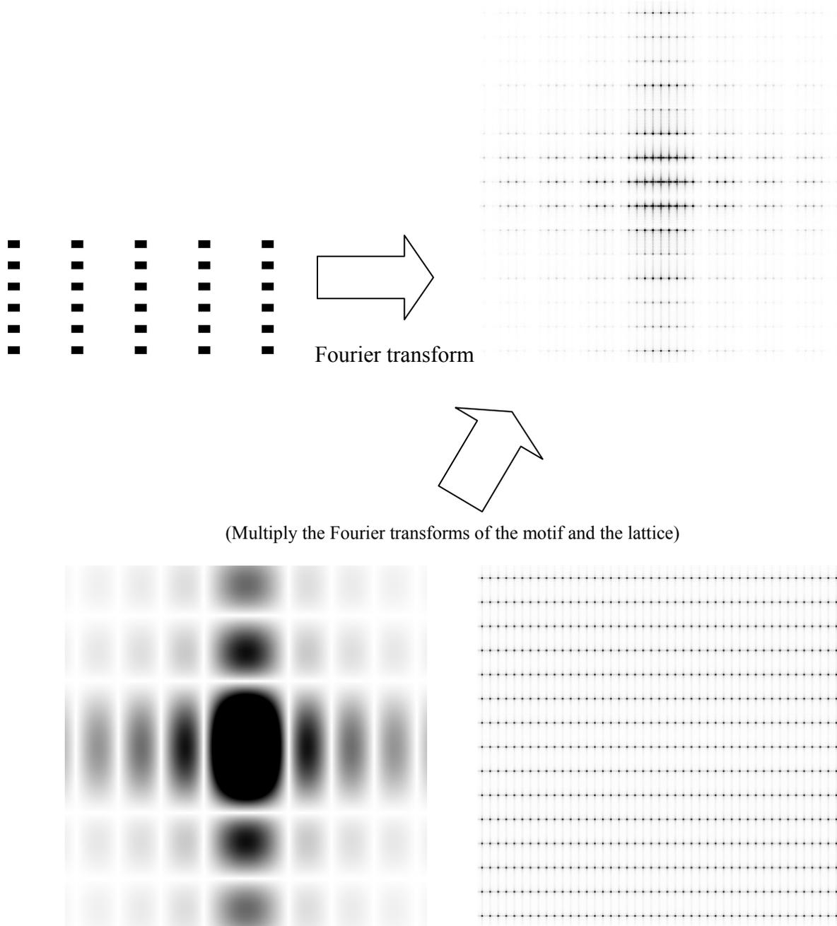
Figure 6 – 4: The Fourier transform of the lattice of rectangles is shown in the upper right hand corner. It is the product of the Fourier transform of the rectangle and the Fourier transform of the lattice.
